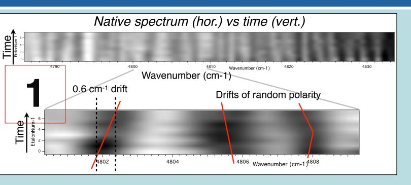
**1. A PROBLEM: PSF DRIFT** A chief limitation to Doppler radial velocity precision is irregular drift of the spectrograph focal spot point spread function (PSF). Here is drift of Mt. Palomar Hale telescope echelle NIR Triplespec vs time (vertical). Note nasty random polarity and magnitude of drift vs position along dispersion axis.
