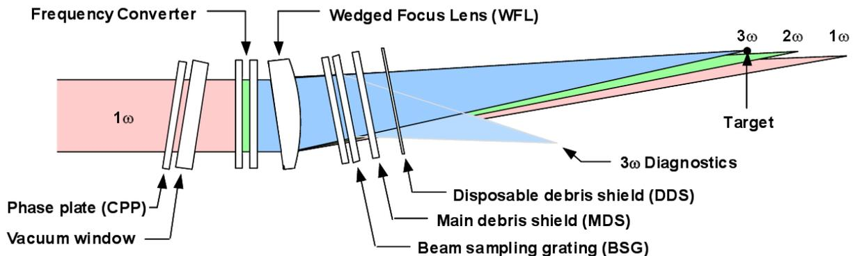
Figure 2. Final optics assembly (FOA) schematic
