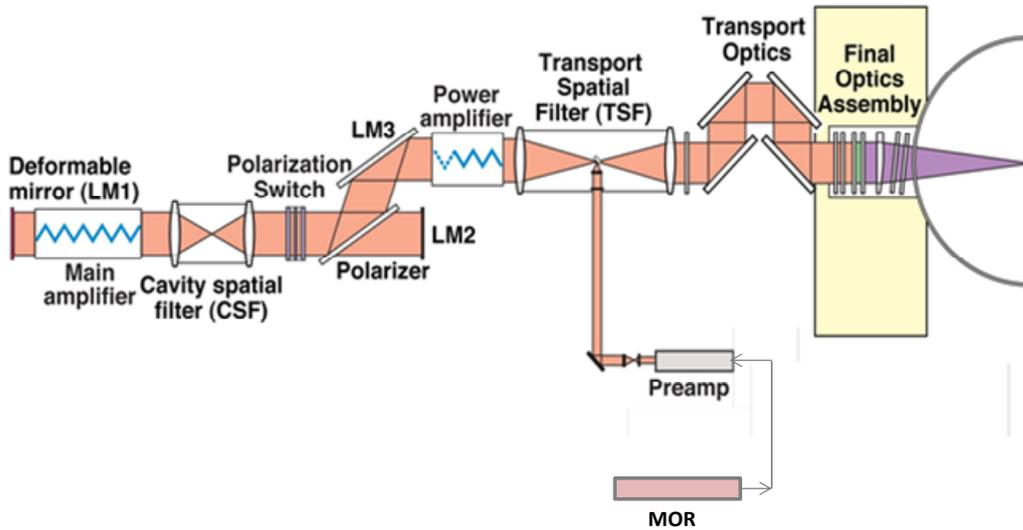
Figure 1. A beam path from start to finish
