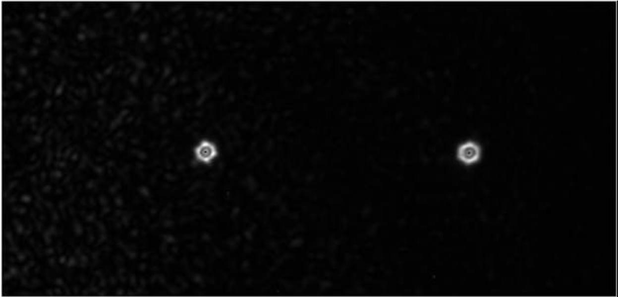
Figure 3. FOA corner cube reflected beam image
