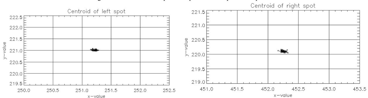
Figure 7. Scatter plot of left and right fiducial of FOA corner cube image
