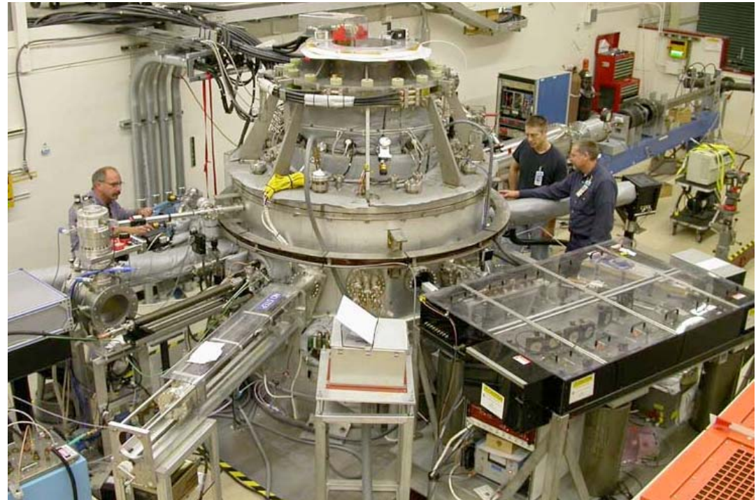
The SSPX facility at Livermore showing the vacuum vessel and major external diagnostics. Not shown: magnet supplies, capacitor banks, and control systems.
