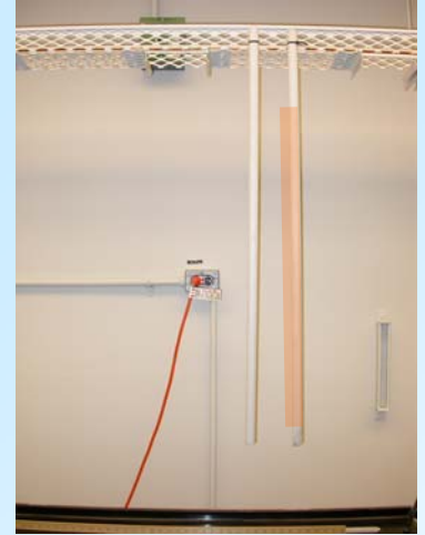
Detailed view of the region where an Eu-152 line source (1 m long) was hidden in the right pipe
