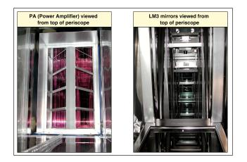
The LOIS inspection system for the Main Laser has mirrors, relay optics and intervening glass. Light scattering sites can still be detected
