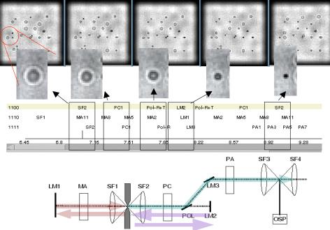
FRODO (based on ICE GDM<sup>\*</sup>) was able to find diffraction rings on NIF Final Optics by tuning 4 adjustable parameters
