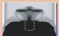
Back-lit fast x-ray image (above) and HYDRA computer simulation (below) of a supersonic (70,000 mph) aluminum plasma jet through aerogel 22 ns after a two-beam laser ablation pulse. The experiment was performed by LLNL, LANL and AWE in the National Ignition Facility (NIF).
